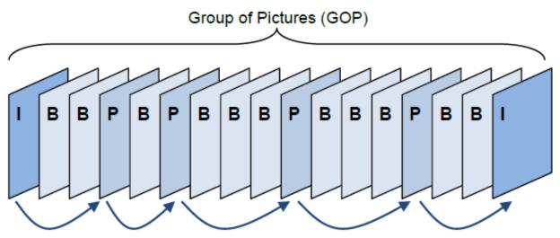
The Intra 'I' frame contains a complete picture. Each Predictive 'P' frame encodes the difference from the previous 'P' or 'I' frame. Bidirectional 'B' frames add more efficiency but also require more computational power and are not normally used in IP CCTV.
